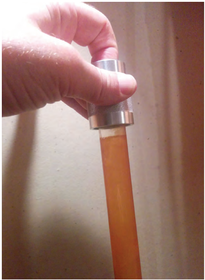
Make sure that the ultraviolet light bulb sleeve is cleaned on a regular basis. If the sleeve is dirty, the ultraviolet rays cannot properly inactivate the germs in the water, allowing contaminated water to flow through untreated.
